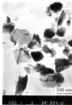
Figure 2. TEM image of nanocrystalline SnS 2 as in Figure 1.
